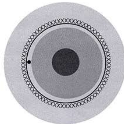
鋁箔及銅網編織隔離電纜 Aluminum Foil / copper braid shield
